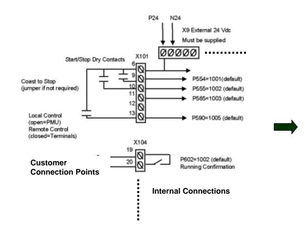
Step 1: Dry set of contacts between terminals X101, pin#6 and pin#13 for Local/Remote Mode Selection. Jumper if not required.
